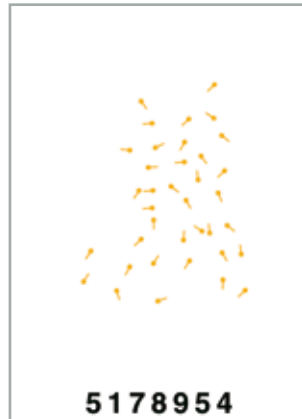
The minutiae are transformed via an algorithm and stored as a reference template.
