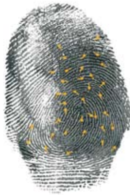
Digital image of a fingerprint showing the minutiae recognized and used by the system.
